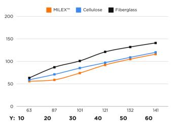
**Vertical Axis**: Temperature of Insulation Material **Y Axis**: Time in Minutes in Oven at 200 °F
